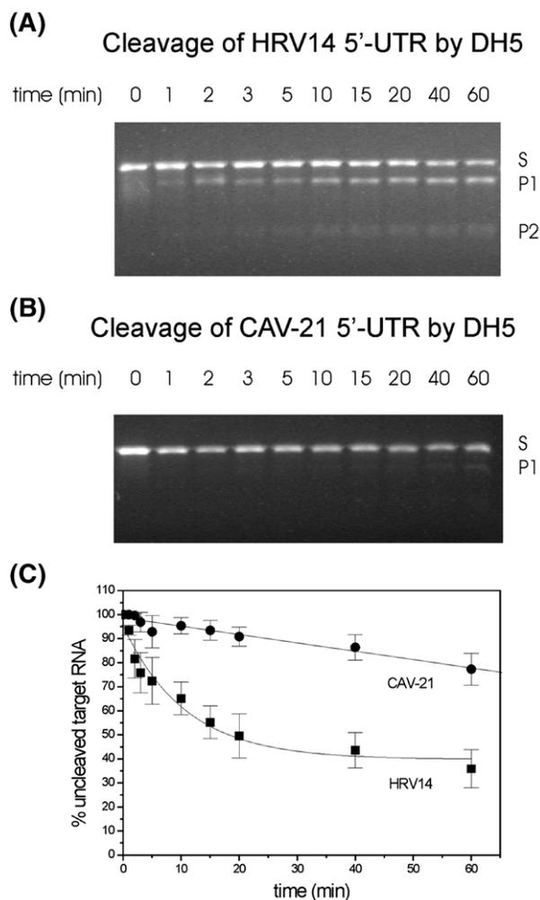
**Figure 2.** Time-course of the cleavage of *in vitro* transcribed 5' UTRs of HRV14 (A) and CAV-21 (B) by unmodified DNAzyme DH5 under single turnover conditions. S, uncleaved substrate; P1 and P2, product bands. (C) Comparison of the cleavage of the 5' UTRs of HRV14 (squares) and CAV-21 (circles) by unmodified DH5. Exponential fit of the mean of three independent experiments.
